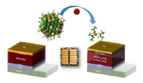
Remote doping of colloidal quantum-dot solar cells by altering their lightharvesting (left) or hole-transporting layer (right). Credit: KAUST
