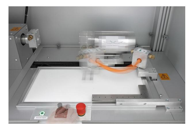
The system sets the bending radius to realistic values matching those encountered in vehicle applications. Credit: Fraunhofer-Gesellschaft
