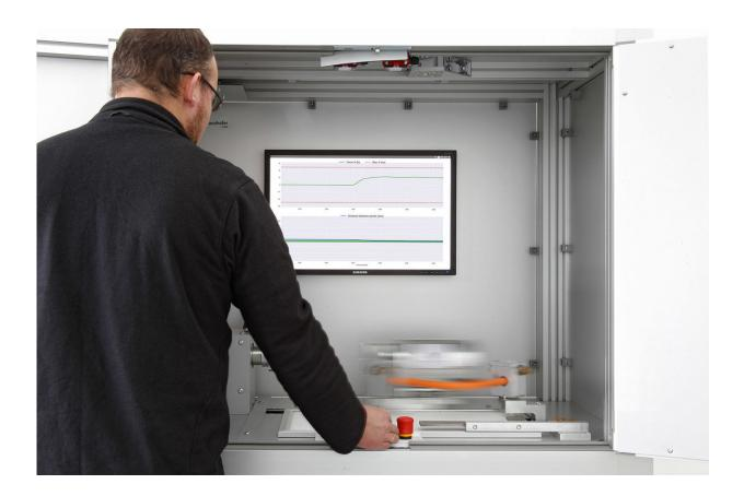
The tests run automatically – all the user needs to do is clamp in the cable and press the start button. Credit: Fraunhofer-Gesellschaft
