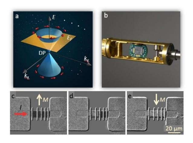
Figure: (a) Schematic diagram illustrating the Dirac cone of topological insulator and spin-momentum locking. (b) Topological insulator/ferromagnet (Bi2Se3/NiFe) spin-orbit torque devices. (c-e) Magneto-optic Kerr effect (MOKE) images of highly efficient spin-orbit torque driven magnetization switching in Bi2Se3/NiFe by a pulsed current at room temperature and zero
