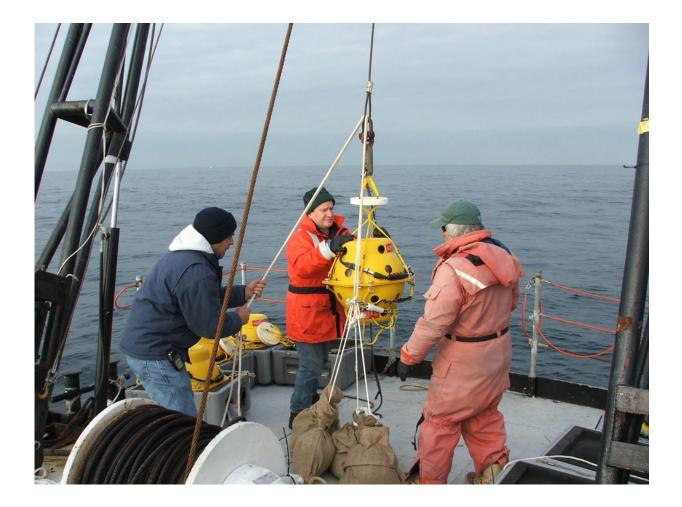
Marine Autonomous Recording Units (MARUs) like this one, being deployed off the coast of Massachusetts, were among the five types of listening devices used during the study to record right whale sounds. The MARU is moored to the ocean floor and fully submerged, recording ocean sounds around the clock before it pops to the surface on command so the data can be retrieved and
