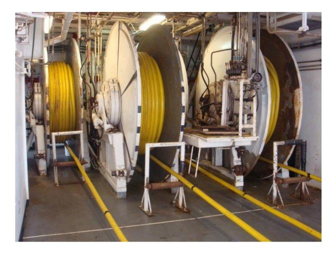
Rolls of seismic streamers. The researchers used very long seismic streamers -reaching almost five miles long -- to image the seafloor using soundwaves. Credit: Shoushou Han/ UT Austin.
