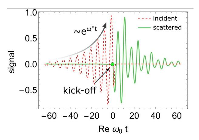
Virtual absorption effect in a thin layer of a transparent material. The dotted line indicates the amplitude of a time-dependent incident wave; the solid line is the amplitude of a scattered signal that comprises both incident and transmitted waves. The scattered signal is absent up to t=0, suggesting that the incident wave energy is perfectly "locked" in the layer. Image courtesy of the researchers. Credit: MIPT
