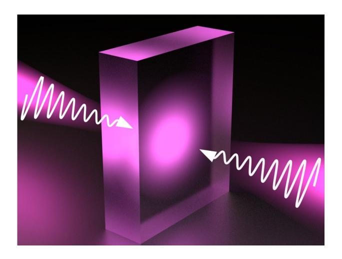
Schematic of a virtual light absorption process: A layer of a transparent material is exposed to light beams from both sides, with the light intensity increasing in time. Image courtesy of the researchers. Credit: MIPT
