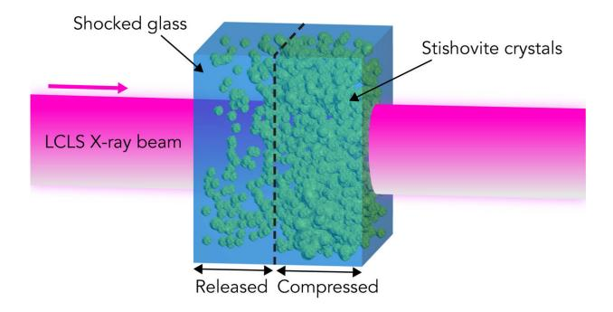
This drawing depicts the process that turns silica into shocked glass after it's hit with a shock wave like one from a meteor impact. At right, compression has transformed the silica into stishovite crystals. On the left, the compression has been released and the stishovite crystals have transformed into shocked glass. The LCLS X-ray laser beam recorded this process, which happens within 30 nanoseconds. Credit: A.E. Gleason et al., Nature Communications
