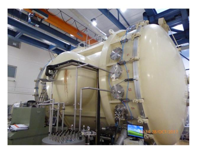
ESA's Aeolus satellite is sealed in the thermal vacuum chamber at the Centre Spatial de Liège in Belgium to make sure it will work in space. The satellite will measure profiles of the world's winds using novel laser technology. This will not only advance our knowledge of atmospheric dynamics, but also provide muchneeded information to improve weather forecasts. Credit: European Space Agency
