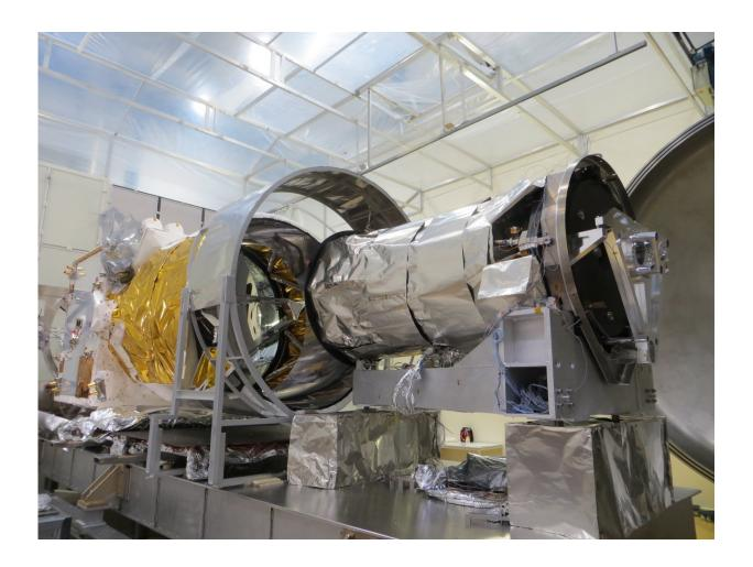
ESA's Aeolus satellite ready to be put in the thermal—vacuum chamber for testing. Simulating the environment of space, the chamber is used to make sure the satellite will work in space. Aeolus will measure profiles of the world's winds using novel laser technology. This will not only advance our knowledge of atmospheric dynamics, but also provide much-needed information to improve weather forecasts. Credit: European Space Agency
