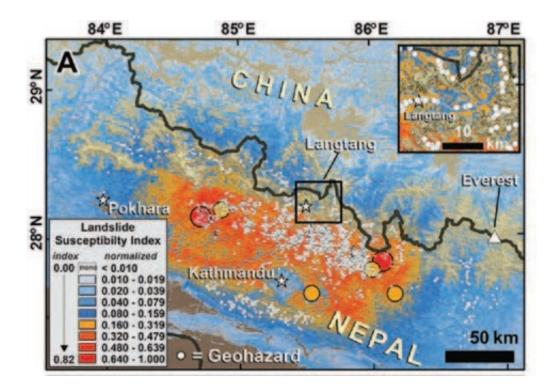
Debris landslide susceptibility with mapped hazards (white dots). Susceptibility inunits of acceleration divided by g (9.81 m/s2). Credit: NASA
