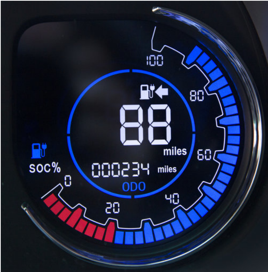
The speedometer of the Chanje V8070 electric medium-duty truck is displayed, Thursday, Nov. 2, 2017, in New York. The vehicle can carry a load of up to 6,000 pounds for a distance of about 100 miles on a single charge. (AP Photo/Mark Lennihan)
