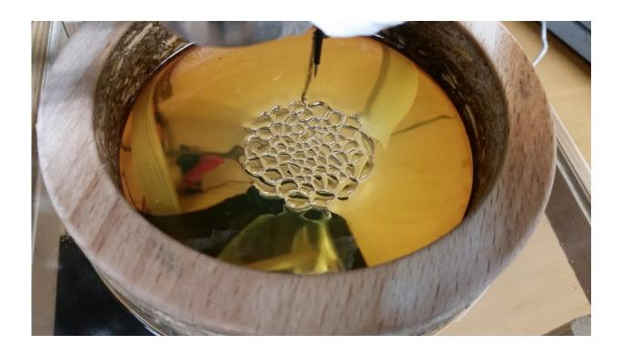
Figure from "The Electric Honeycomb; an investigation of the Rose window instability"
