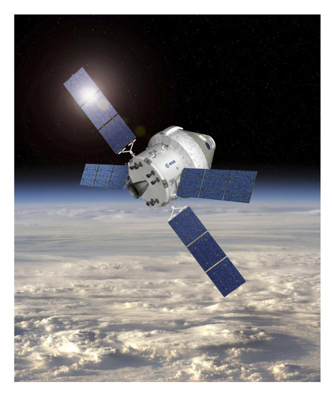
An artist's impression of the Orion crew capsule with ESA's service module. The module sits directly below the capsule and provides propulsion, power, thermal control, and water and air for four astronauts. The solar array spans 19 m and
