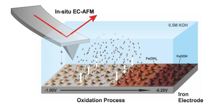
Schematic of the measuring method: the tip of the in situ electrochemical atomic force microscope scans the surface of the iron electrode. Laser-beam deflection reveals spatial irregularities, which can be compared to each other over the course of several cycles. Credit: Forschungszentrum Jülich / H. Weinrich
