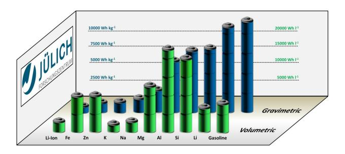
Gravimetric and volumetric energy densities of various metal-air battery systems in comparison with Li-ion batteries and conventional gasoline. Credit: Forschungszentrum Jülich / H. Weinrich
