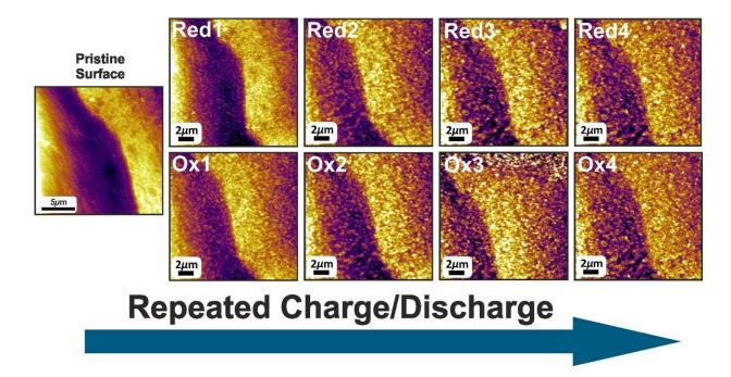
Diagram of changes to the electrode surface over the course of four charging/discharging (redox) cycles. Credit: Forschungszentrum Jülich / H. Weinrich
