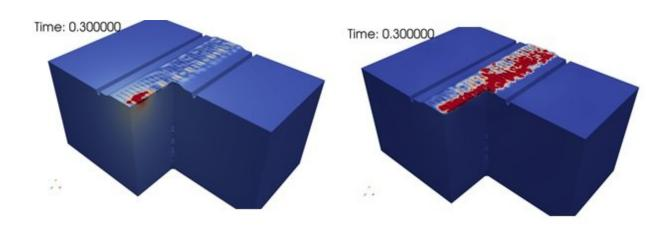
Amplitude of the displacement field after a train passes on the track. The left-hand figure corresponds to a simulation with homogeneous ballast and the right-hand image to a simulation with heterogeneous ballast. Credit: Lucio de Abreu Corrêa, Laboratoire de Mécanique des Sols, Structures et Matériaux (CNRS/CentraleSupélec)
