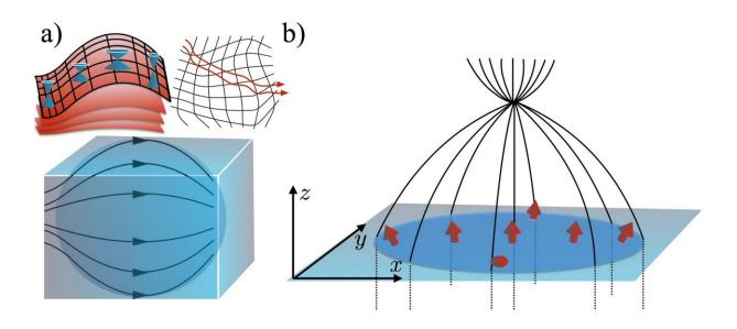
(a) By local manipulation of material parameters, it is possible to tune the properties of charge carriers in Weyl semimetals; (b) With suitable local manipulation of material parameters, one can tailor the carrier motion and design novel electronic devices such as the electron lens, which focuses the incoming carriers. Credit: Academy of Finland
