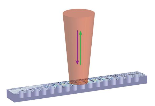
The coupled device between the photonic crystal nanobeam cavity and perovskite nanocrystals, which overlays with the cavity mode profile. The arrows indicate that the excitation and generated signal are coupled in and out of the device vertically. Credit: Zhili Yang, University of Maryland
