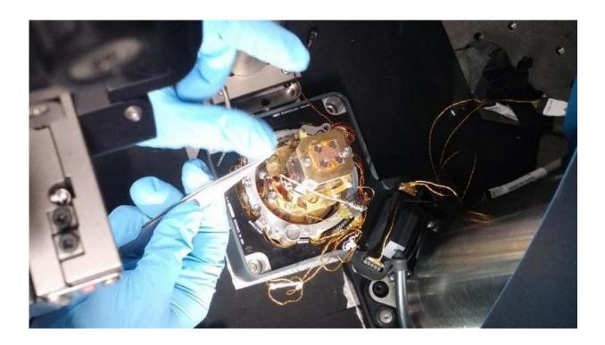
A cryogenic sample chamber, with diamond sample mounted on copper cold plate. Credit: Yoav Romach
