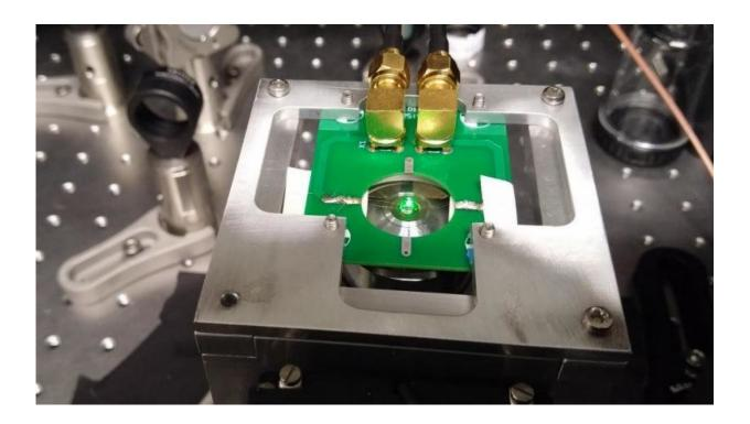
A diamond sample illuminated by green light in custom-built microscope. The sample is placed on a special mount, within a printed circuit board, used to deliver microwaves which allow quantum manipulations and magnetic sensing with the NVs. Credit: Yoav Romach
