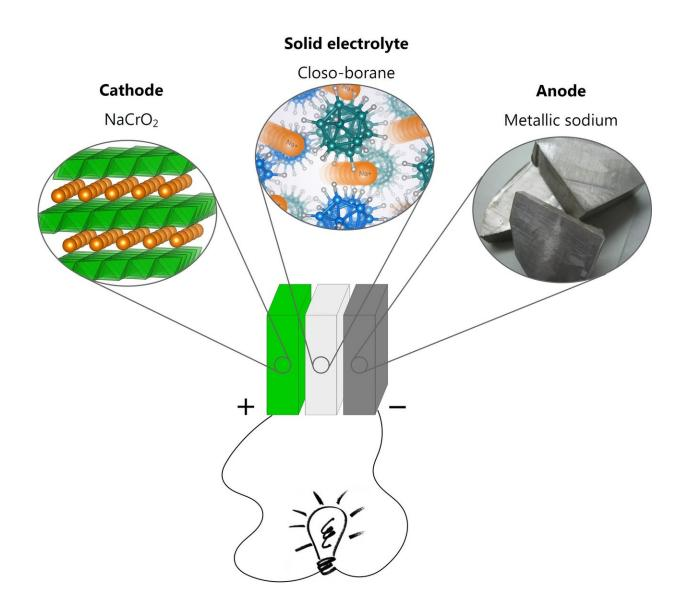
Diagram of the composition of the solid sodium battery. Credit: Empa
