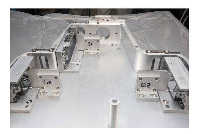
The three spectrometer channels inside the instrument. Credit: Elle Starkman
