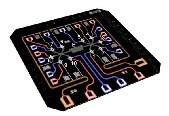
False-color circuit image showing 10 superconducting qubits (star shapes) interconnected by a central bus resonator B (gray). Credit: Song et al. ©2017 American Physical Society
