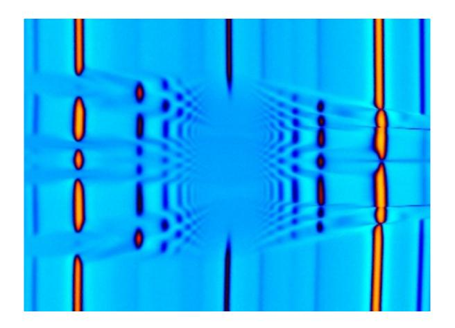
Capacitance measurement of bilayer graphene at a high magnetic field. The vertical dark blue to orange lines are signatures of fractional quantum Hall states that are shared between the two layers of the bilayer graphene sheet. The vertical line going through the center is believed to host an intriguing type of particles: non-Abelian anyons. Credit: University of California - Santa Barbara
