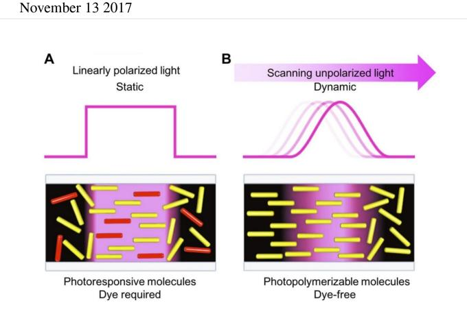
A represents the molecular alignment through conventional photoalignment methods. B represents the molecular alignment achieved through the currently reported scanning wave photopolymerization method. Credit: Atsushi Shishido, Tokyo Institute of Technology
