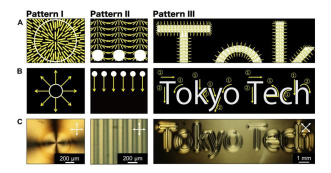
A represents a schematic illustration of the desired patterns of alignment. B represents irradiated light patterns of expanding toroid shapes, periodic dots, and the words Tokyo Tech. C represents POM images under crossed polarizers. Credit: Atsushi Shishido, Tokyo Institute of Technology
