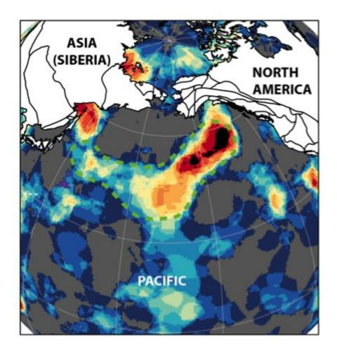
Seismically imaged relics of subducted oceanic plates (warm colors surrounded by dashed green line) that reveal that subduction was once active in the northern Pacific. The island arc was sitting above these subducted oceanic plates at this time, and it later collided with northeast Asia. Credit: CEED
