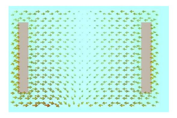
Simulated surface currents on a slotted microstrip patch with illumination of a silicon superstrate. Credit: University of Bristol
