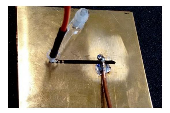
4.2GHz – 6 GHz optically tunable cavity backed slot antenna. Silicon samples can be seen in the slot and an optical fibre is being held in place over one sample for tuning. Credit: University of Bristol
