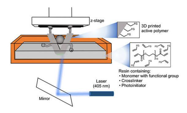
Catalysts can be built in one step by directly shining a laser through a bath of customized resins that polymerize and harden layer-by- layer. Credit: Ames Laboratory
