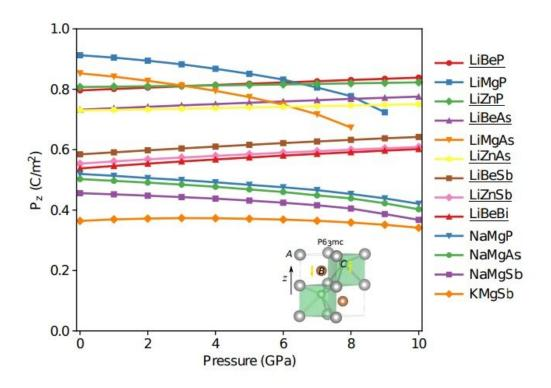
A comparison of ferroelectric materials, some of which exhibit the negative longitudinal piezoelectric effect. Materials with pressure-enhanced ferroelectricity are underlined. Credit: Liu et al. ©2017 American Physical Society
