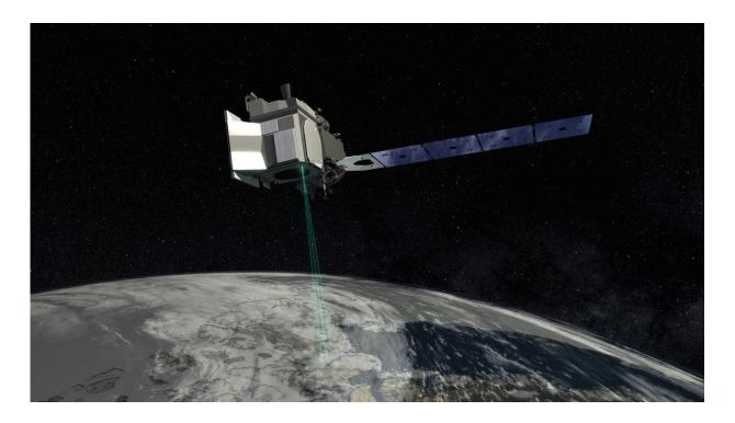
ICESat-2 (illustrated here), slated to launch in Fall 2018, will measure the height of Earth's surface from space. Credit: NASA
