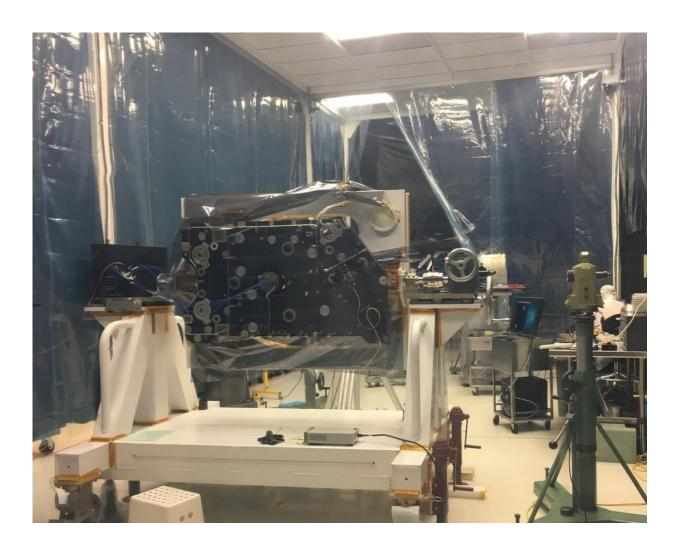
The GEDI instrument, which is designed to capture the vertical structure of
