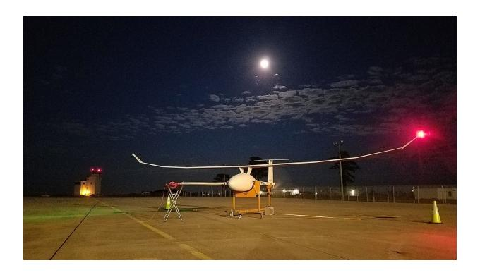
The VA001 can carry 35 pounds of payload, flying at 500 to 15,000 feet above sea level. Its primary attraction -- and the primary reason NASA funded its development through the SBIR program -- is its ability to carry out research over some of the most forbidding locations on Earth. Credit: Jeremy Novara/Vanilla Aircraft
