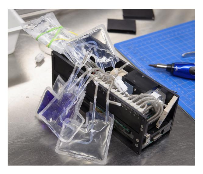
EcAMSat contains this experimental module, inside which the E. coli are stored. Nutrients, the antibiotic, a special dye and waste are stored in bags connected through a series of tubes to the microfluidics card – a device storing small pools of liquid containing the bacteria. Credit: NASA/Ames Research Center/Dominic Hart
