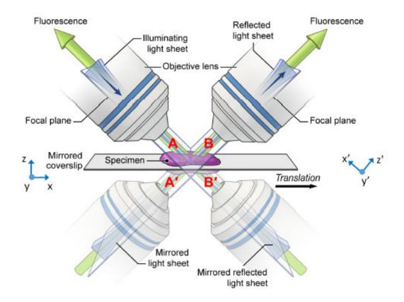
In this diagram, you can see how the mirrored coverslip allows for four simultaneous views. Credit: Yicong Wu, National Institute of Biomedical Imaging and Bioengineering
