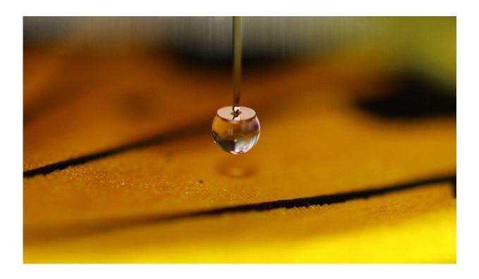
The droplet probe of the microscope on a superhydrophobic golden birdwing (Troides aeacus) butterfly wing. Credit: Matti Hokkanen / Aalto University
