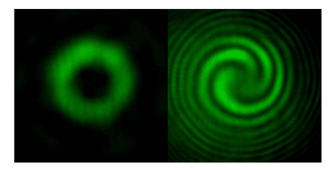
A metasurface can generate strange new beams of light that swirl and corkscrew. The black hole in the center of these vortices can be used to image features smaller than half a wavelength of light or move tiny molecules. Credit: Capasso Lab/Harvard SEAS
