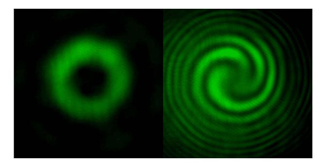
A metasurface can generate strange new beams of light that swirl and corkscrew. The black hole in the center of these vortices can be used to image features smaller than half a wavelength of light or move tiny molecules. Credit: Capasso Lab/Harvard SEAS
