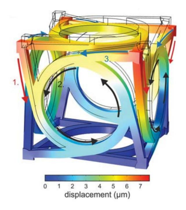
Calculated deformed cell and displacement under uniaxial loading. The arrows aid the discussion of the mechanism: 1. The arms connecting the corners with the rings move downward. 2. This motion leads to a rotation of the rings. 3. This rotation exerts forces onto the corners in the plane normal to the pushing axis, resulting in an overall twist of the unit cell around this axis. Credit: (c) *Science* (2017). DOI: 10.1126/science.aao4640
