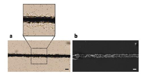
Using a one-step laser fabrication process, researchers created flexible hybrid microwires that conduct electricity. (a) An optical microscope image of the silver (black) and silicone (clear) microwires. (b) Scanning electron microscopy image of the same fabricated structure. Both scale bars are equal to 25 microns. Credit: Mitsuhiro Terakawa, Keio University
