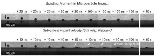
Above-critical impact velocity (805 m/s): Adhesion
