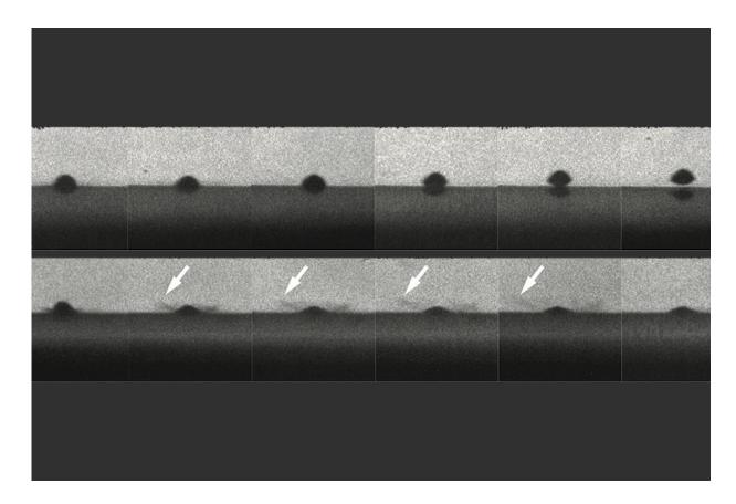
The top row of photos shows a particle that melts the surface on impact and bounces away without sticking. The bottom row shows a similar particle that does not melt and does stick to the surface. Arrows show impact sprays that look like liquid, but are actually solid particles. Credit: Massachusetts Institute of Technology
