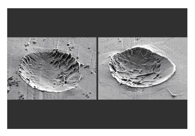
Micrographs of a metal surface after impact by metal particles. Craters are formed due to melting of the surface from the impact. Credit: Massachusetts Institute of Technology
