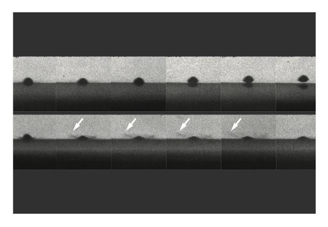
The top row of photos shows a particle that melts the surface on impact and bounces away without sticking. The bottom row shows a similar particle that does not melt and does stick to the surface. Arrows show impact sprays that look like liquid, but are actually solid particles. Credit: Massachusetts Institute of Technology
