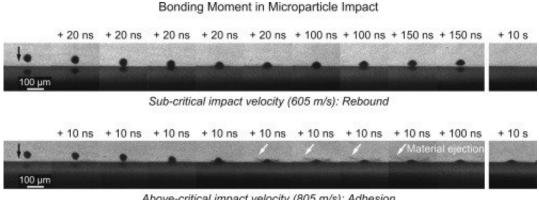
Above-critical impact velocity (805 m/s): Adhesion
