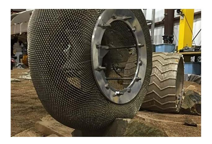
The Mars Spring Tire being tested at NASA GRS' Slope lab. Credit: NASA/JPL
