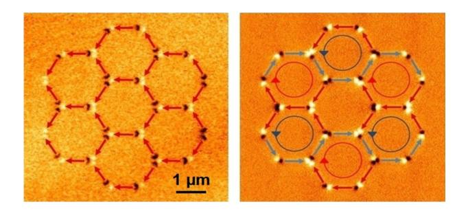
'Hexagonal artificial spin ice ground state' -- a pattern never demonstrated before. Colored arrows show north or south polarization. Credit: Gartside et al/Imperial College London
