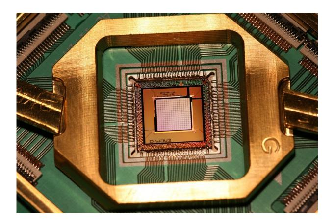
A photograph of D-Wave's 1000+ qubit computer chip under development. CfA scientists and their colleagues have proposed a new way to use photons of light instead of silicon chips as qubits, opening the door to new technologies. Credit: Google
