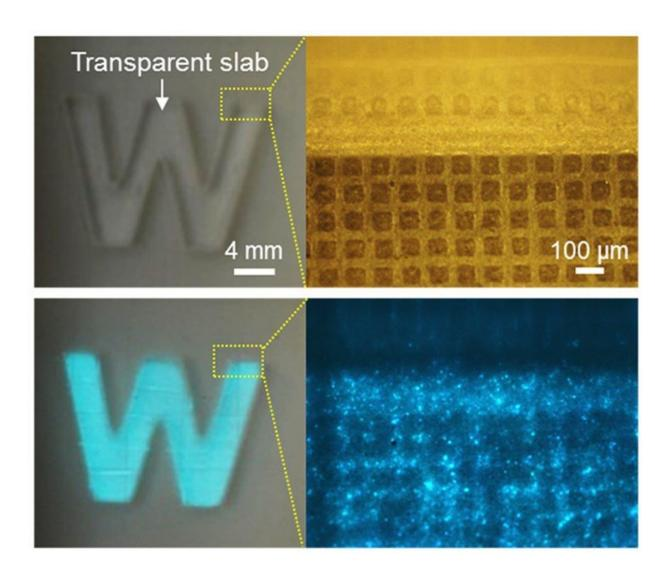
An electronic skin glows when a transparent 'W' is pressed onto it, and a voltage is applied (bottom). Credit: The American Chemical Society
