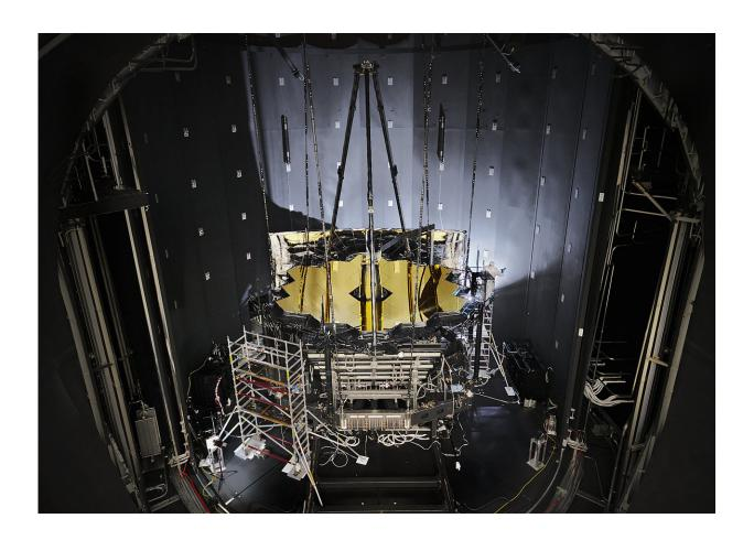
NASA's James Webb Space Telescope sits inside Chamber A at NASA's Johnson Space Center in Houston after having completed its cryogenic testing on Nov. 18, 2017. This marked the telescope's final cryogenic testing, and it ensured the observatory is ready for the frigid, airless environment of space. Credit: NASA/Chris Gunn
