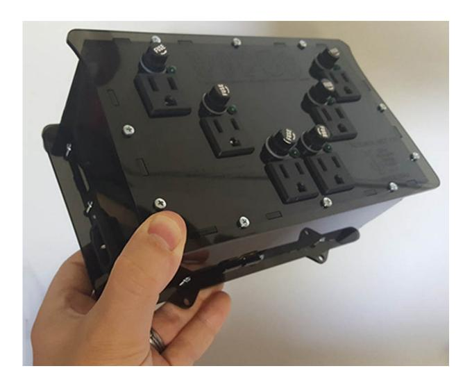
The cy.PIPES system could help virtual reality/augmented reality developers synchronize tools that create environmental conditions like heat or wind. CyUtil LLC, a startup launched by Chauncey Frend of IU's Advanced Visualization Lab, is commercializing the system. Credit: Indiana University
