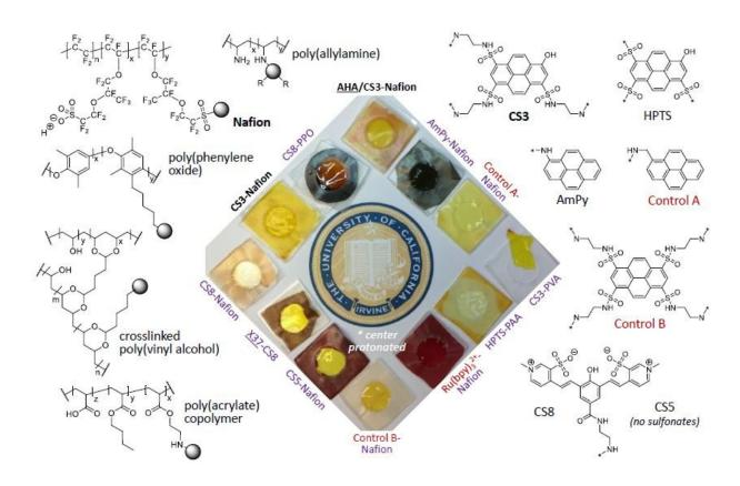
Summary of membrane designs for ionic electricity generation. Credit: Ardo et al.
