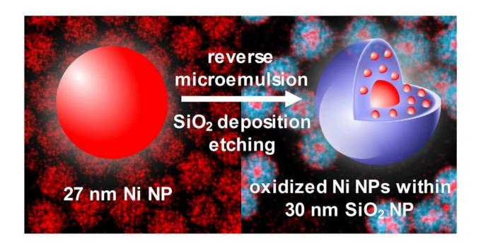
During deposition of a silica shell onto Ni nanoparticles, they are etched, oxidized, and embedded in the silica, which stabilizes the structure during oxidation and reduction. Credit: Brian Lynch. Reproduced by permission of The Royal Society of Chemistry.
