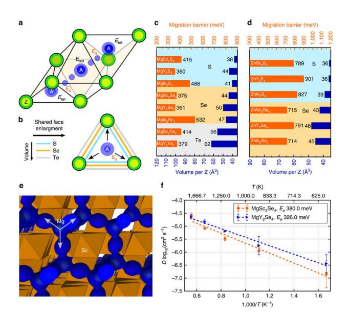
First-principles Mg and Zn migration barriers in sulfides, selenides, and tellurides AX2Z4 spinels (with A = Mg or Zn). a tet–oct–tet migration path in
