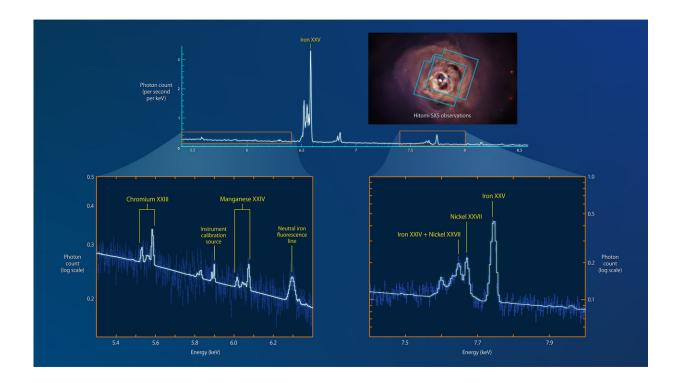
Hitomi's Soft X-ray Spectrometer (SXS) instrument captured data from two overlapping areas of the Perseus galaxy cluster (blue outlines, upper right) in February and March 2016. The resulting spectrum has 30 times the detail of any previously captured, revealing many X-ray peaks associated with chromium, manganese, nickel and iron. Dark blue lines in the insets indicate the actual Xray data points and their uncertainties. Credit: NASA's Goddard Space Flight Center
