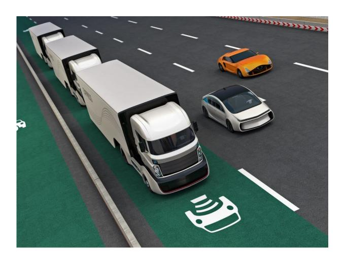
Truck platooning involves a lead truck with a driver guiding other trucks through vehicle to vehicle communication. Credit: cheskyw / 123rf.com, Author provided
