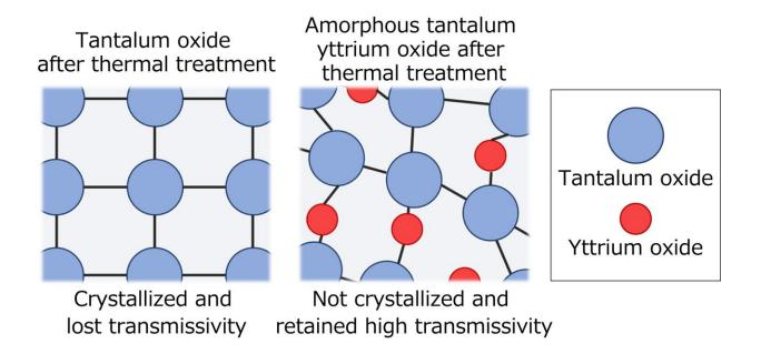
Schematic views of atomic/molecular distribution in tantalum oxide and amorphous tantalum yttrium oxide. Even after thermal treatment at high temperature, amorphous tantalum yttrium oxide remains uncrystallized and retains the random distribution of atoms/molecules, which allows high transmissivity to be maintained. Credit: Toyohashi University Of Technology.
