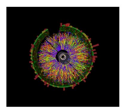
This animation shows a series of collision events at STAR, each with thousands of particle tracks and the signals registered as some of those particles strike various detector components. It should give you an idea of how complex the challenge is to reconstruct a complete record of every single particle and the conditions under which it was created so scientists can compare hundreds of millions of events to look for trends and make discoveries. Credit: Brookhaven National Laboratory
