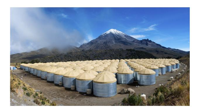
The HAWC Observatory, perched next to a volcano at an altitude of 13,500 feet, uses its 300 massive water tanks to scoop up the products of high-energy particle collisions happening in the upper atmosphere. Credit: Jordan Goodman
