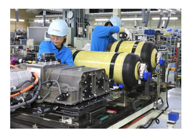
In this Oct. 30, 2017, photo, workers of Toyota Motor Corp. set hydrogen-stored tanks, in yellow, to be placed into a Mirai fuel cell vehicle at the automaker's Motomachi plant, in Toyota, western Japan. Toyota is banking on a futuristic "electrification" auto technology called hydrogen fuel cells for its zero-emissions option. The Associated Press got a tour of Toyota's Motomachi plant that assembles the Mirai fuel cell vehicle. (AP Photo/Yuri Kageyama)
