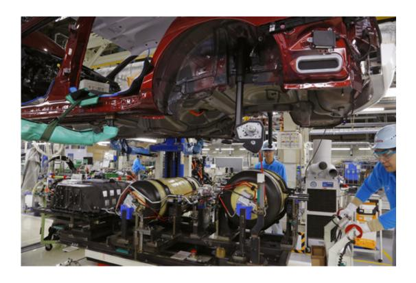
In this Oct. 30, 2017, photo, workers of Toyota Motor Corp. assemble a Mirai fuel cell vehicle at the automaker's Motomachi plant in Toyota, western Japan. Toyota is banking on a futuristic "electrification" auto technology called
